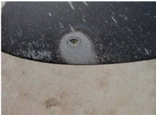
Strong Lightning Strike on a Composite Blade Tip
